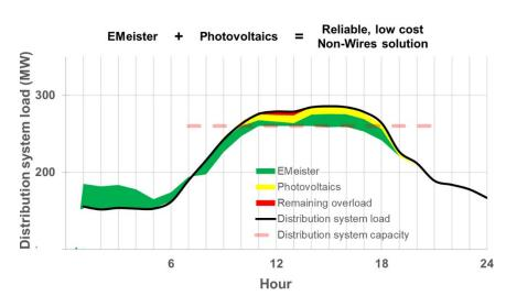
Important ... EMeister unloaded the substation as a byproduct of reducing commercial building electric expense ... and, by definition, ConEd distribution system peak loads occurs on days when PV performs best.
